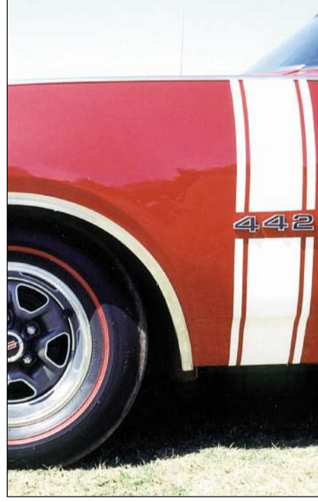
After Pontiac came out with the hot-selling GTO, Olds responded with the numerical designation 442, which stood for "4"-barrel carb, "4"-speed transmission and "2", or dual, exhaust.
